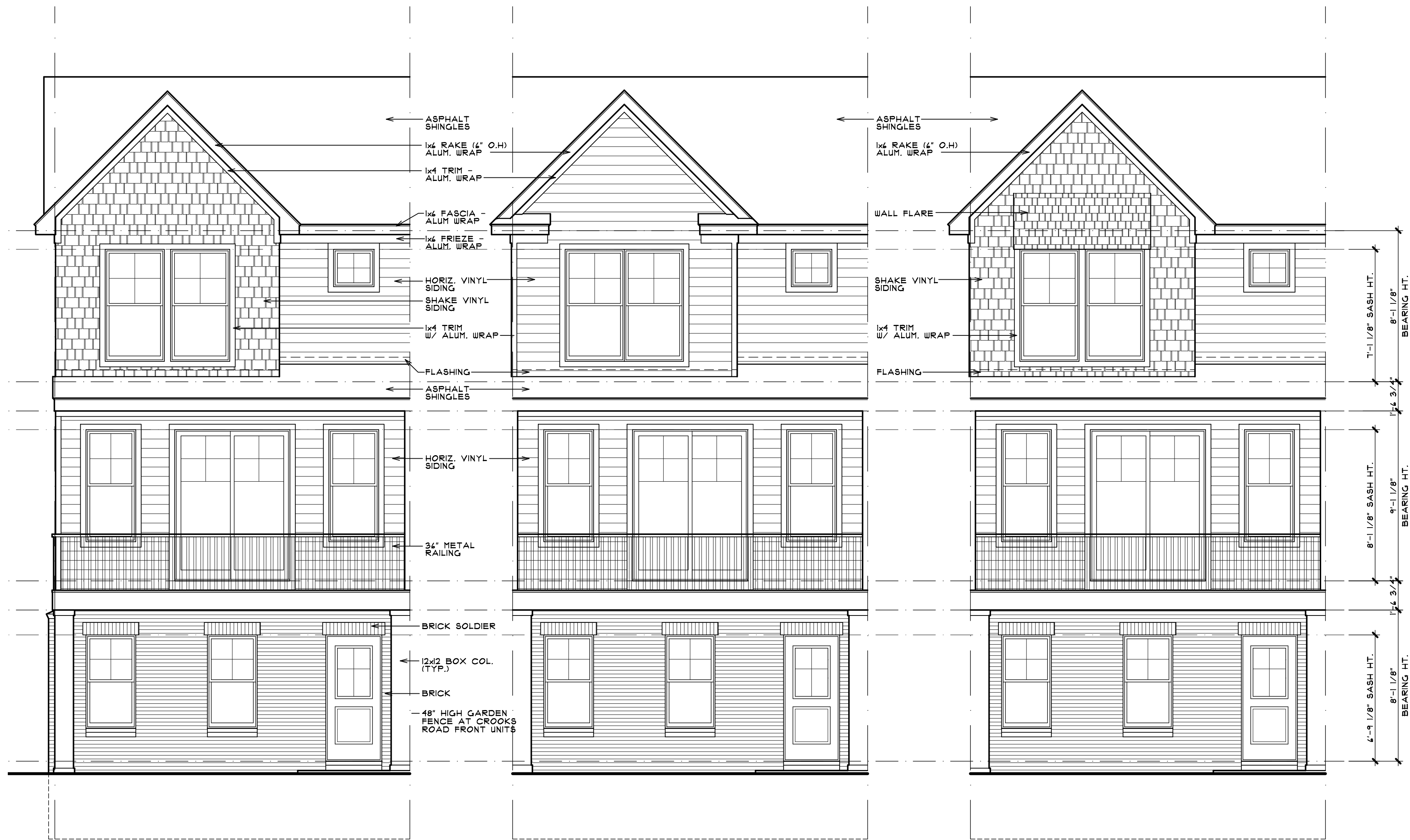
NOTE: ALL WOOD TRIM IS TO BE WRAPPED IN ALUMINUM. ELEVATION 'A' SCALE: 1/4" = 1'-0"
