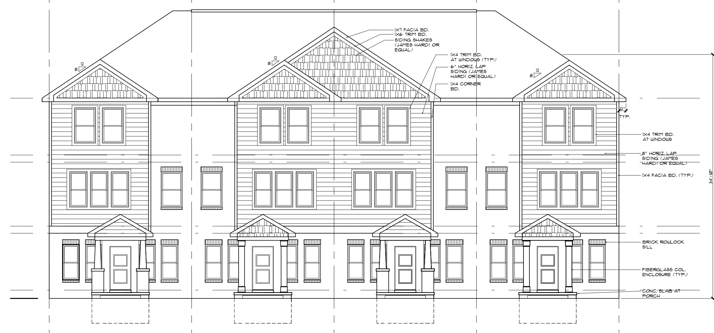
FRONT ELEVATION - 4 UNIT BLDG. 2,300 SF SCALE: 1/4" = 1'-0"
