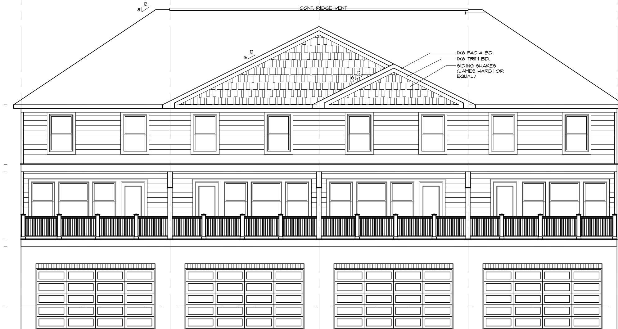
REAR ELEVATION - 4 UNIT BLDG. 2,300 SF SCALE: 1/4" = 1'-0"
