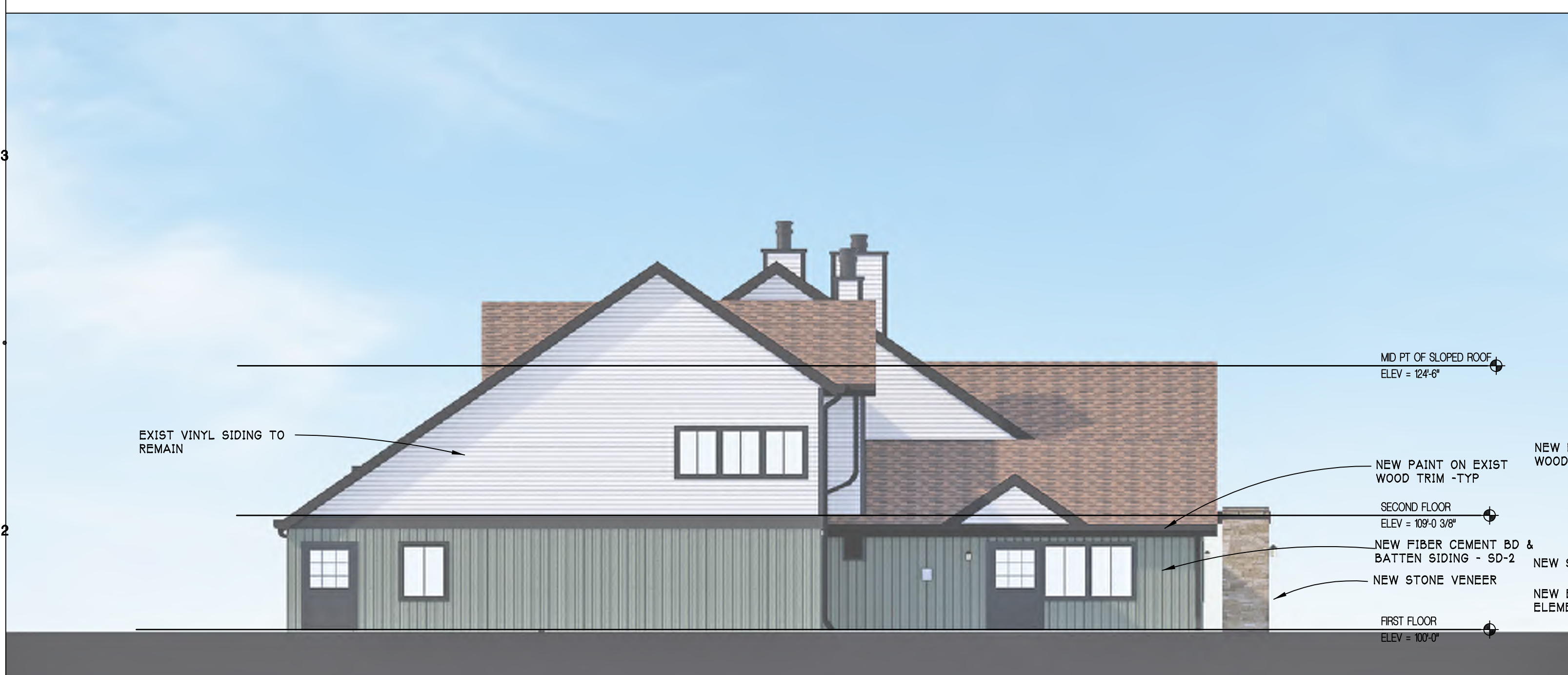
F1 NORTH ELEVATION A-210 SCALE - 1/8" = 1'-0" ELEVATION SHEET
