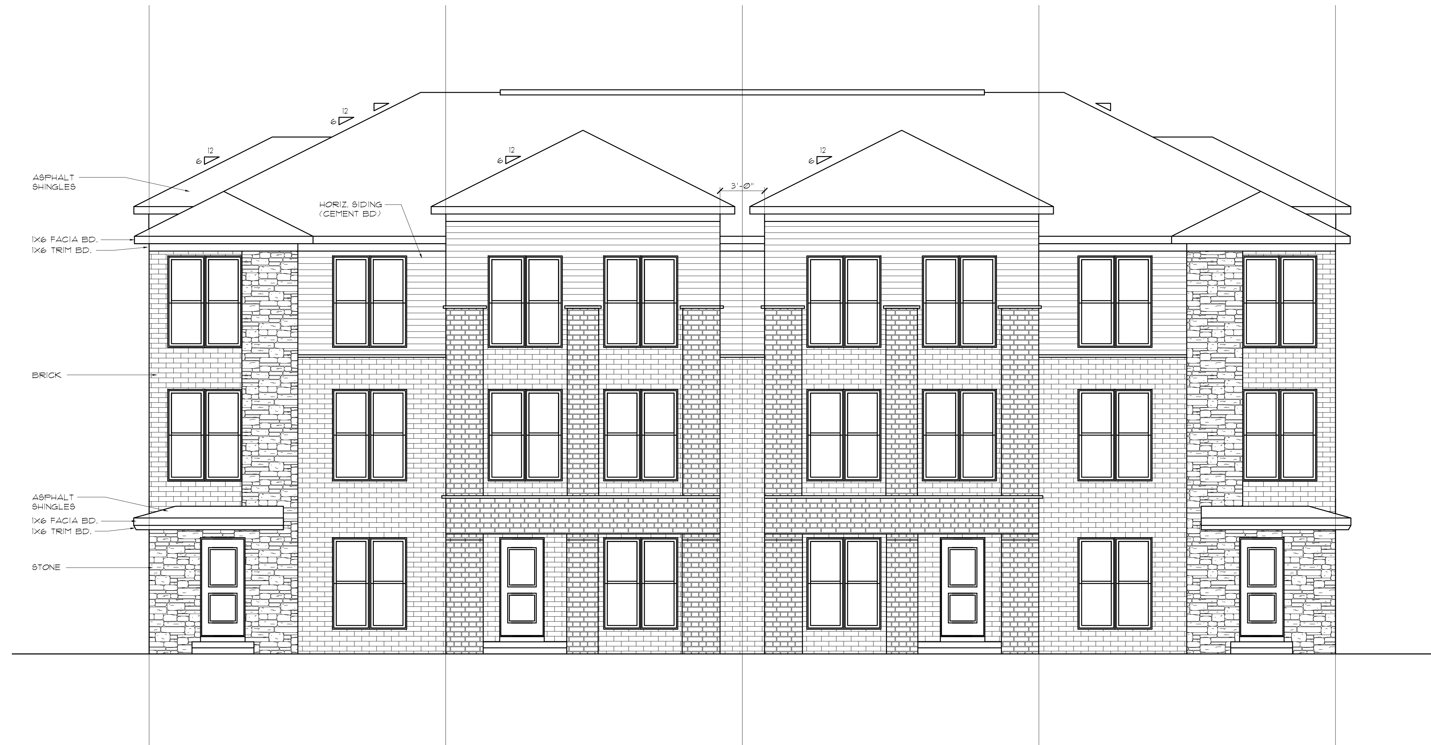
FRONT ELEVATION - 4 UNIT BLDG.
