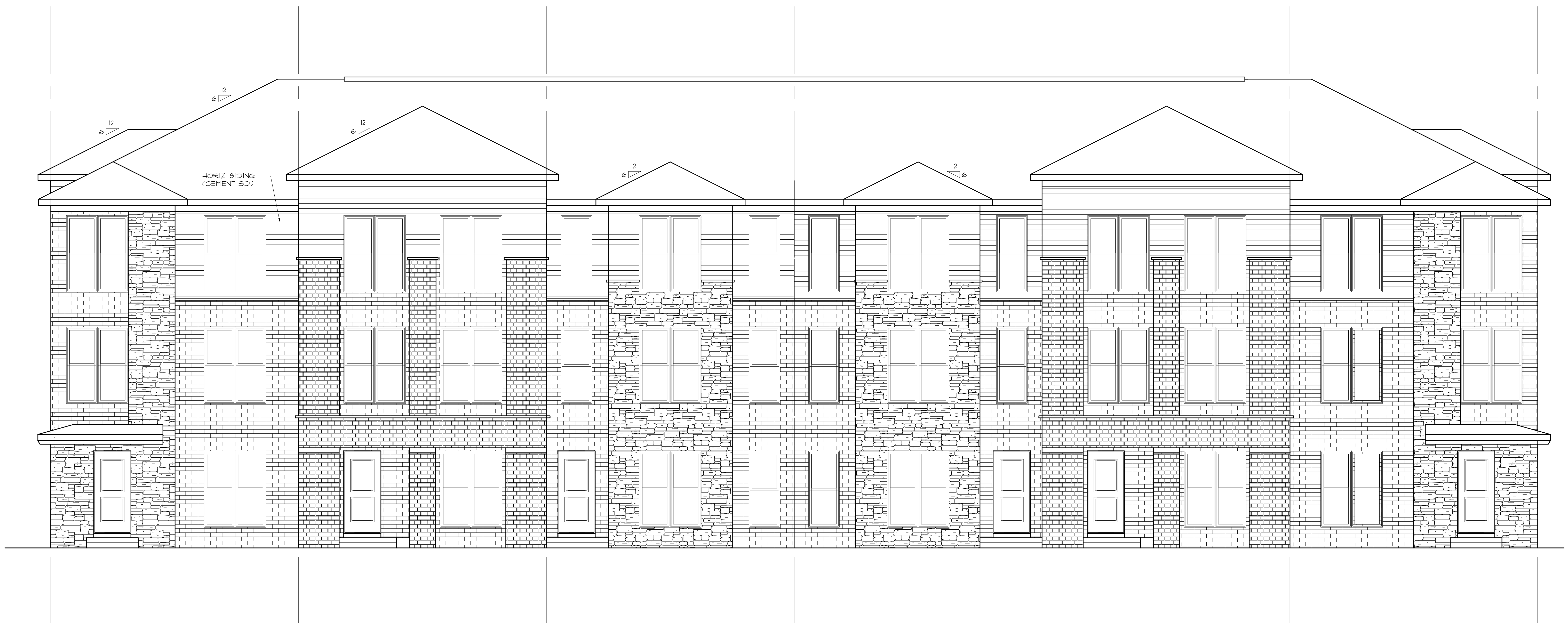
FRONT ELEVATION - 6 UNIT BLDG. SCALE: 1/4" = 1'-0"
