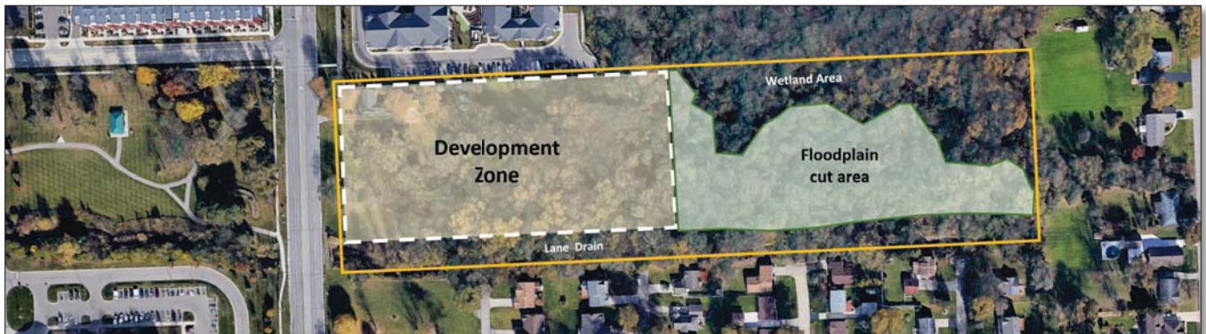
The western portion of the site has been determined to have the characteristics suitable for development, whereas the eastern portion of the site will be reserved for the preservation of the natural features, floodplain cut area, and re-forestation of the wooded areas.
