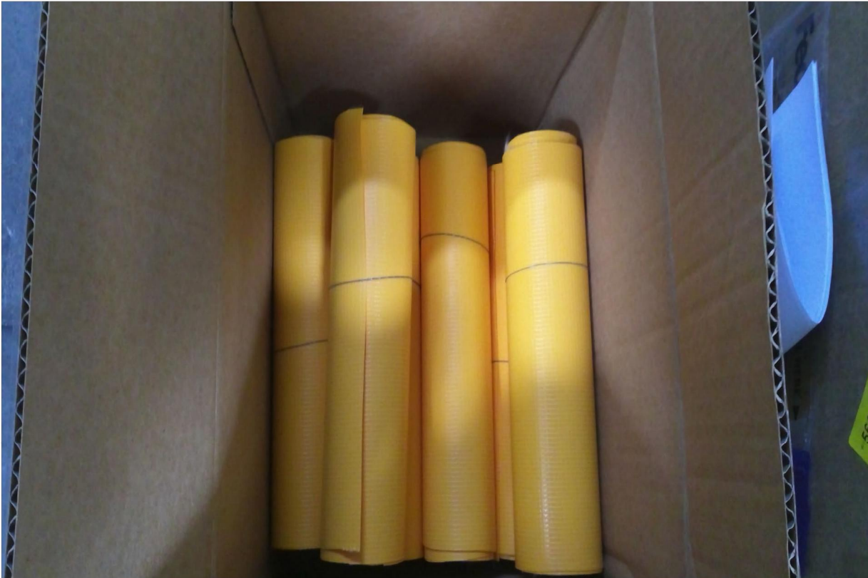
FUNBOX PVC Tarpaulin for Inflatables, nominal thickness 0.0210" as received from client.
