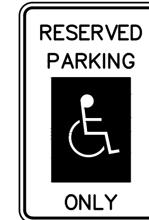
12" x 18" (R7-8) GREEN BORDER AND LEGEND WHITE SYMBOL, BLUE BACKGROUND, REFLECTORIZED DET 2 BARRIER FREE PARKING SIGN DETAIL NOT TO SCALE
