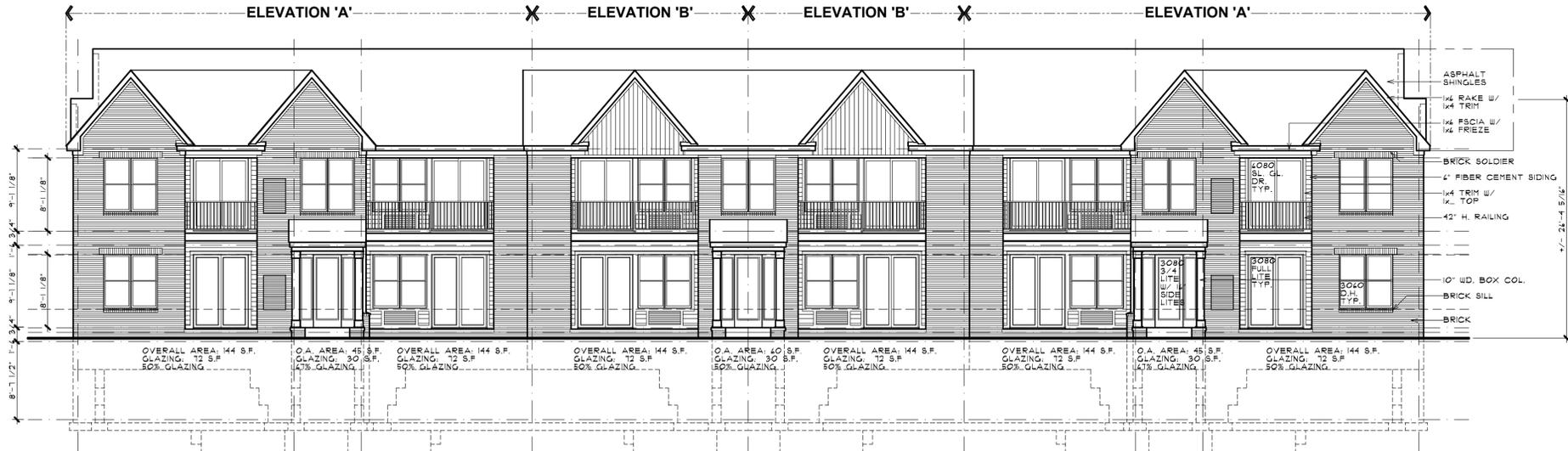
**FRONT ELEVATION - BUILDING TYPE 'A-1'**
