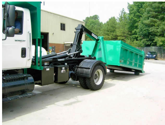
Hook Lift Truck with Various Body Attachments (not actual vehicle, for example only)
