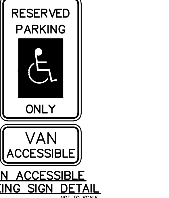
VAN ACCESSIBLE PARKING SIGN DETAIL NOT TO SCALE
