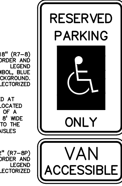
ADA & VAN ACCESSIBLE PARKING SIGN DETAIL (NOT TO SCALE)
