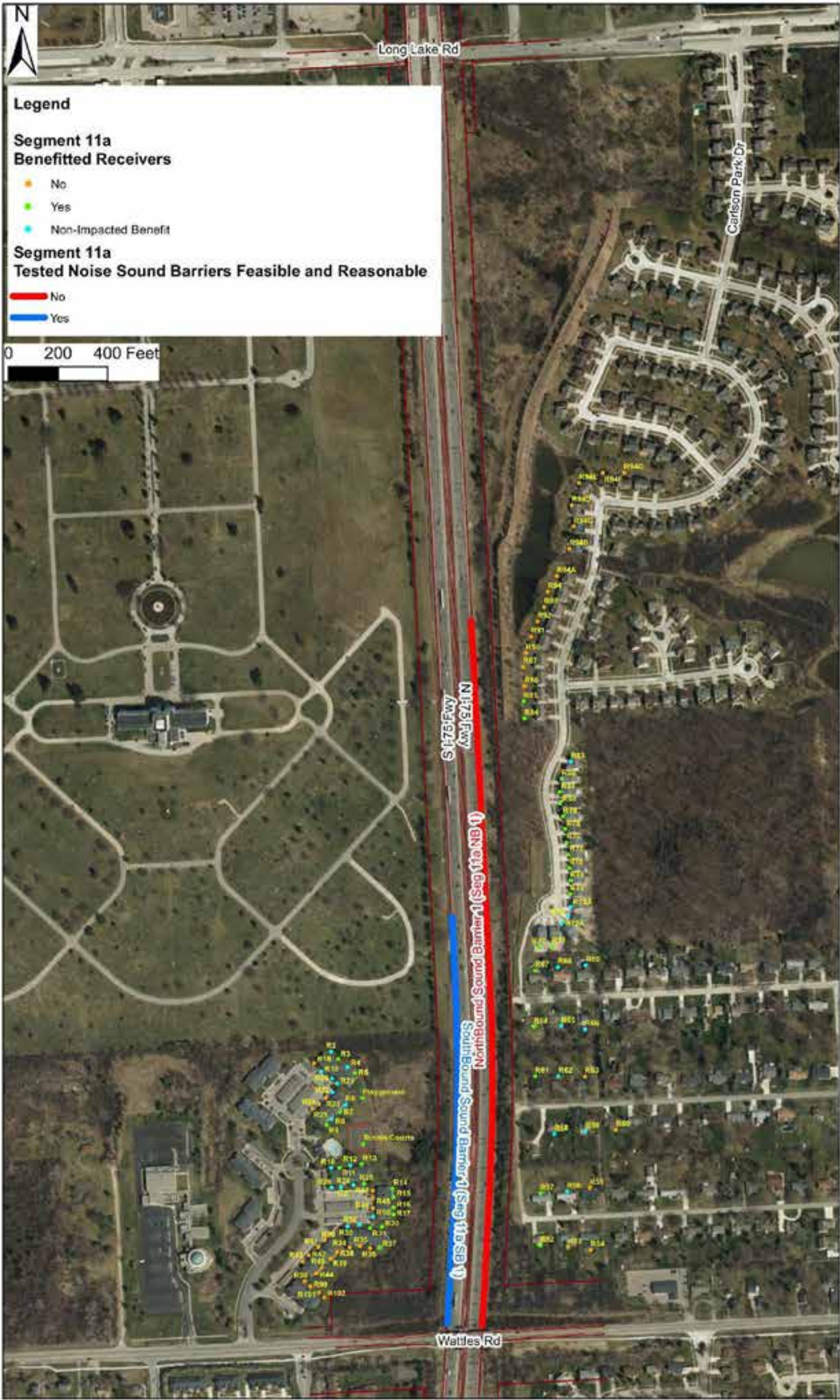
Figure 19 – Segment 11A Sound Barrier Design Configuration for Benefitting Receivers Behind Southbound Barriers SB1 and Northbound Barrier NB1
