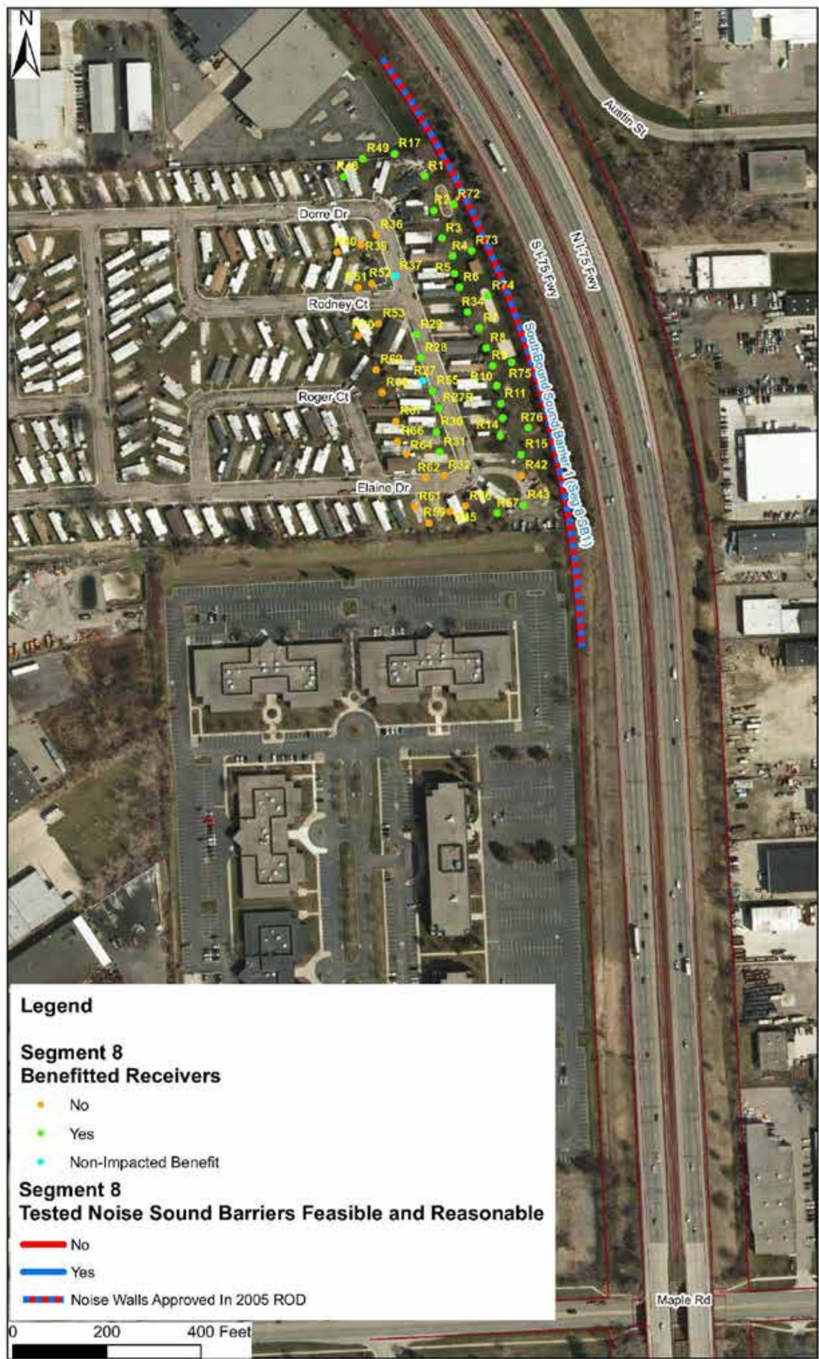
Figure 16 – Segment 8 Sound Barrier Design Configuration for Benefitting Receivers Behind Southbound Barrier (SB1)
