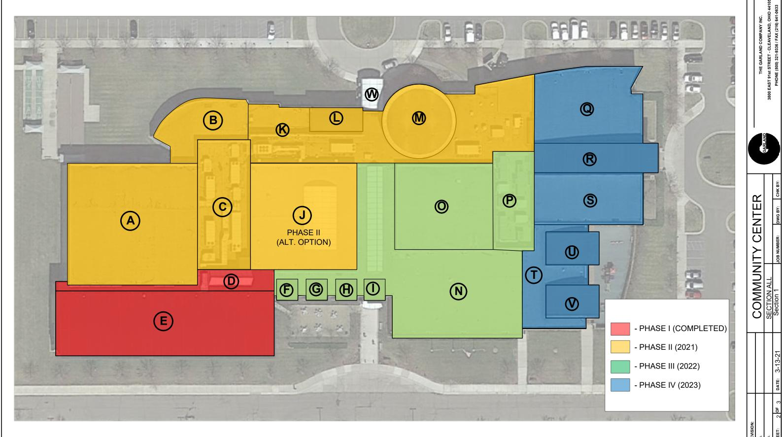
EPDM BASE BID SCOPE: 2-PLY, COLD-PROCESS URETHANE MODIFIED SYSTEM IN ZERO VOC ADHESIVE WITH ALUMINUM COATING
