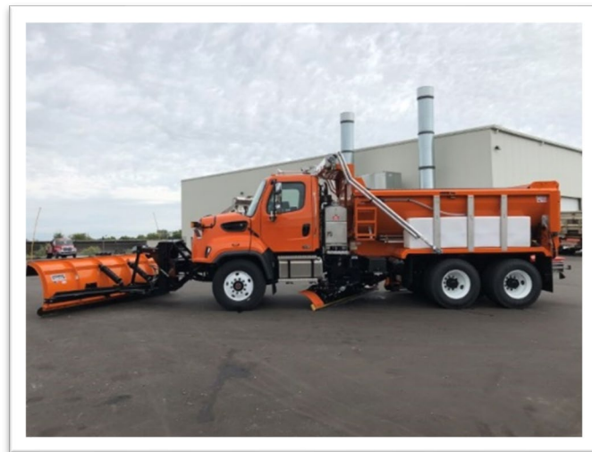
Freightliner Truck with Dump Body & Snow Removal Equipment Installed
